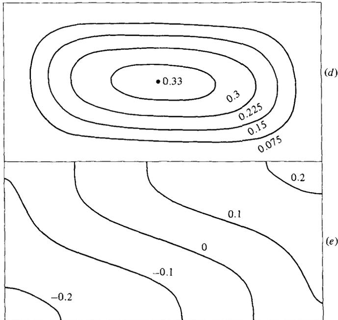
FIGURE 5. The numerical results for run 2,  $Gr = 62.5$ : (a) the variation of  $Nu$  with  $t^*$ ; (b), (c) the flow and temperature fields at the peak in (a),  $t^* = 10$ ; (d), (e) the flow and temperature fields at steady state.  $T^*$  has been normalized by  $T_{\max}^*$ , and the numerical values in (b) and (d) are values of  $\phi/\nu$ . Note the change in timescale.
