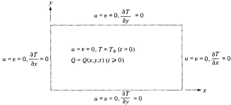
FIGURE 1. The rectangular-cavity notation, boundary and initial conditions.
