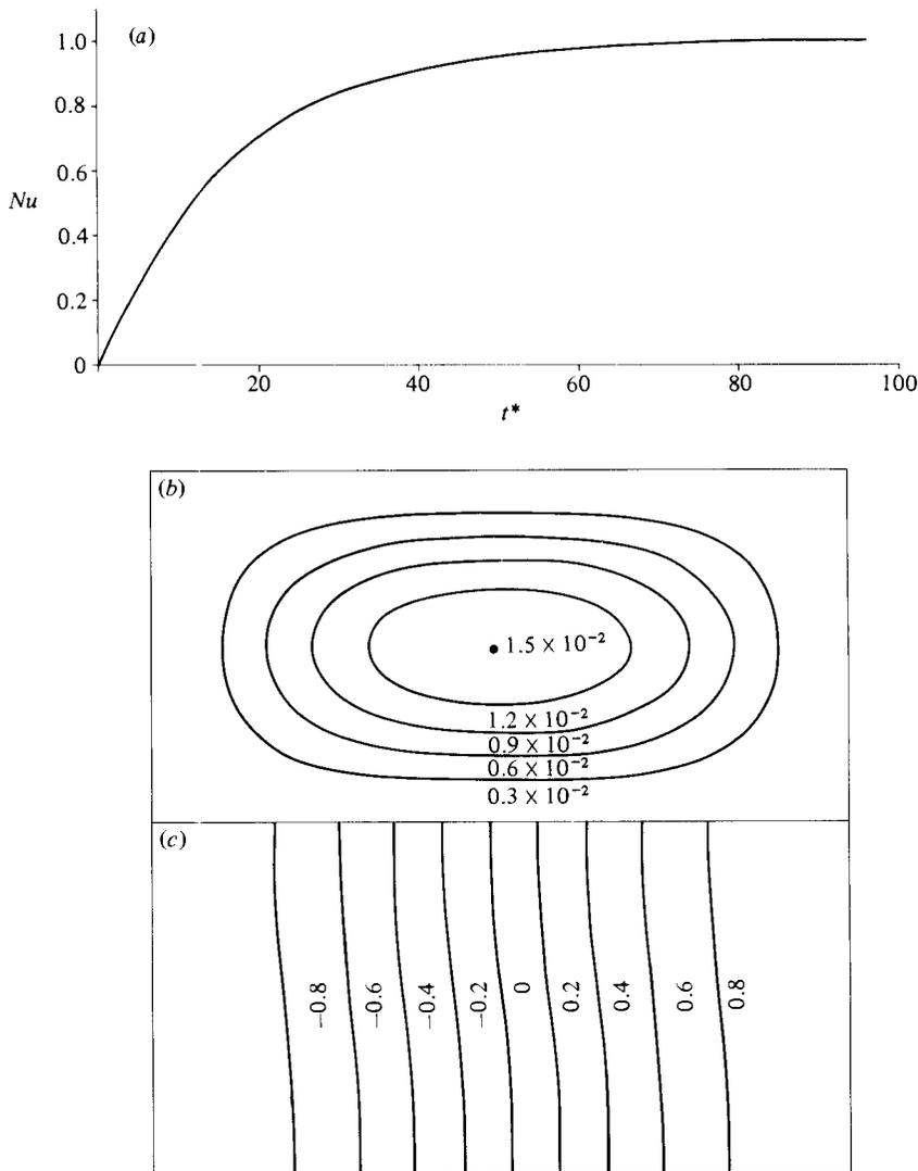
FIGURE 4. The numerical results for run 1,  $Gr = 0.625$ : (a) the variation of  $Nu$  with  $t^*$ ; (b) the steady-state streamlines; (c) the steady-state isotherms.  $T^*$  has been normalized by  $T_{max}^*$ , and the numerical values in (b) are values of  $\phi/\nu$ .
