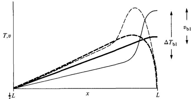
FIGURE 2. An illustration of the adjustments to the temperature and vertical velocity profiles near the wall at the hot end of the cavity. The solid lines are temperature and the broken lines velocity at  $t < t_c$  (heavy) and at steady state (light).
